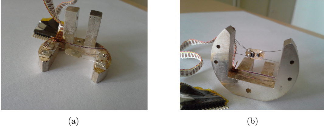
Figure 12: Sample holder for the low-temperature measurements. The top side (a) where the grease and sample is placed on a platform made of silver, and the bottom side (b) with the heater (thin film metal resistor 10 k \Omega ) and thermometer (RuO 2 2.7 k \Omega ). Please note the four wires (Pt0.9Ir0.1) connecting thermometer and heater each to utilize the 4-point probes method.
